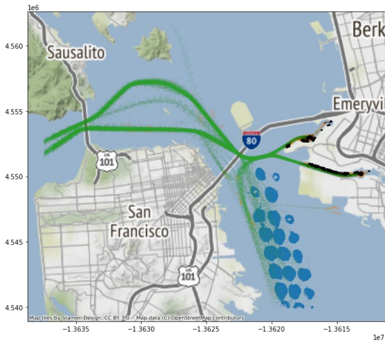
Figure 5: AIS positions of vessels calling at the Port of Oakland in 2015 shown in transit (green), at anchor (blue), maneuvering (orange) and at berth (black).
