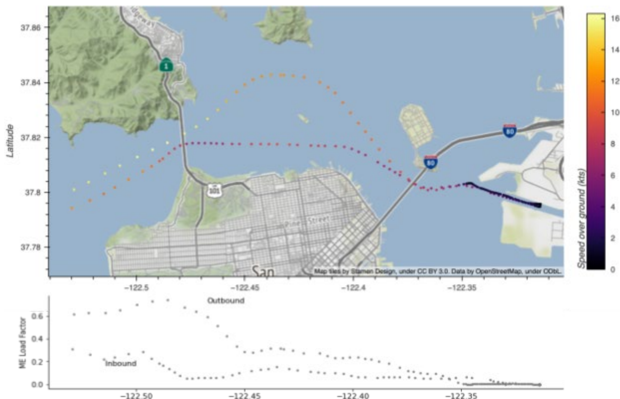
Figure 2: Speed over ground positions and main engine load factor as the MSC Anna calls at the Port of Oakland
